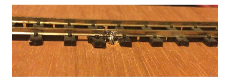
Again the magnification makes it look quite rough, but it's a good join. Notice how the wire is only on the bottom flange of the rail so that if it's on the inner face it won't foul the wheels.
